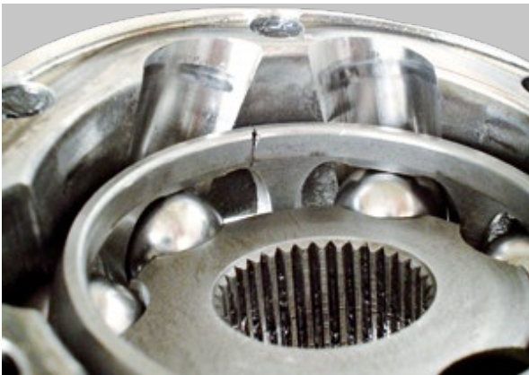
Defective plunging ball joint
