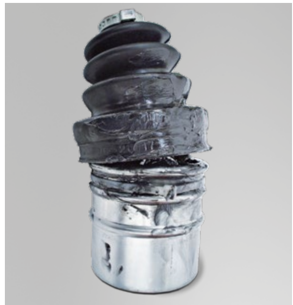
Incorrect fitted boot
