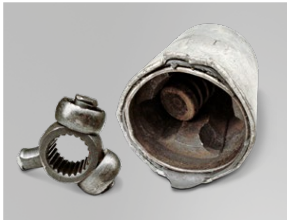
Defective tripod ball joint
