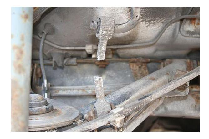
Particular stress is applied on coupling rods and stabiliser mounts on vehicles with lowered suspensions or with broken suspension springs.
